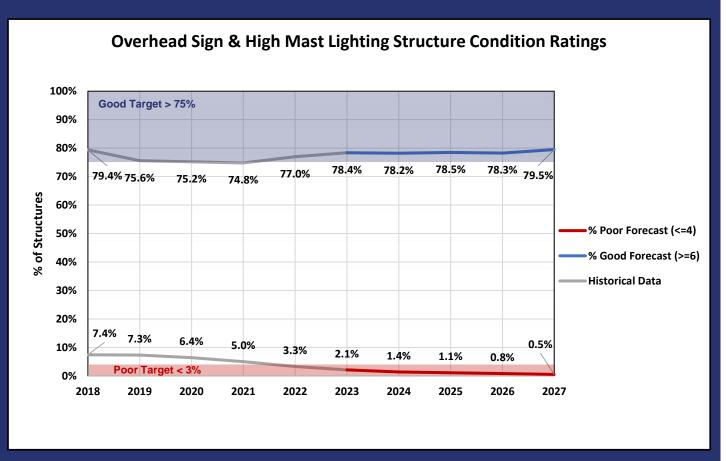
\*Note: The 3-Year Condition Forecast is based on current programmed overhead sign & high mast lighting replacement projects.
